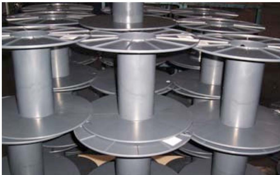
**Figure 8.3: Cable reels successfully moulded using the PP recyclate.**
