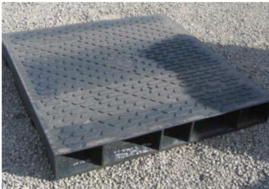
**Figure 8.5: Pallet successfully moulded using the PP recyclate.**
